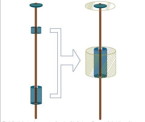
**Fig. 3** Sketch showing the assumption of merging of the feed zones. The outer cylinder is the resulting volume of the forecast
