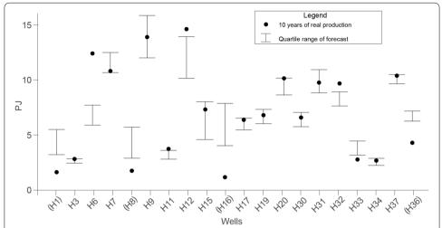
**Fig. 5** Validation of the model given by Eq. (6). The observed value for the extraction is represented as a dot. Forecast using our model with 80% of the data for training is shown as a range whisker. The model is considered to be appropriate when the observed value is inside the range. Wells enclosed in parentheses operated for 22 years and they are not considered for validation as they do not have enough data
