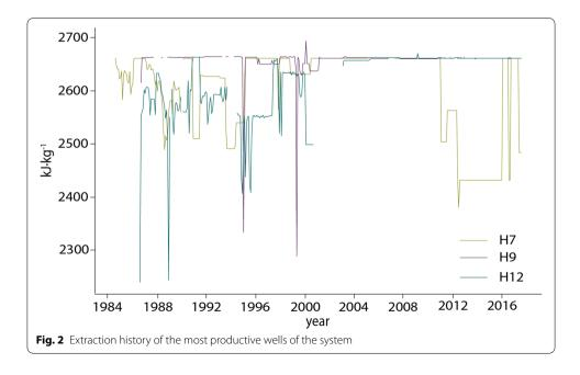
established extraction regime for the next 30 years without any recharge by conduction or convection from below. Furthermore, the initial amount of heat with a sum of the reserve plus the accumulated production of heat is estimated. These two quantities allow the calculation of the heat recovery factor.
