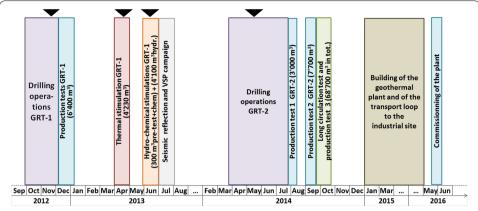
**Fig. 3** Timeline of the operations performed during the development of the Rittershoffen deep geothermal field. The seismogenic periods of interest (during GRT-1 drilling, thermal and hydraulic stimulations and GRT-2 drilling) are indicated by black triangles
