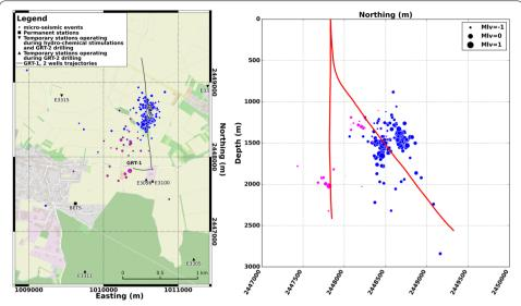
**Fig. 6** Epicenter map (left) and South–North vertical projection (right) of the seismicity recorded during the GRT-1 drilling (magenta circles) and GRT-2 drilling (blue circles)
