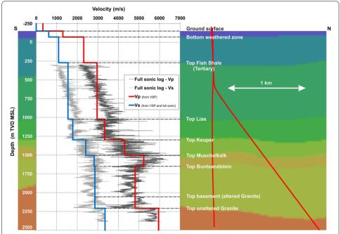
**Fig. 4** Vertical profile of the 3D velocity model along GRT-1 overlaying a vertical South–North section of the 3D P-wave velocity model next to GRT-1 and GRT-2 wells (red curves). The red velocity profile indicates the Vp derived from the VSP, the blue velocity profile indicates the Vs derived from the VSP and the Vp/Vs ratio of the full sonic (see text for further explanations). The Vp and Vs measured by the full sonic log are presented for comparison in dark and light gray, respectively
