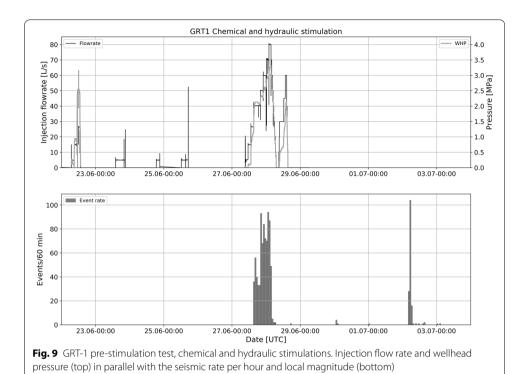
stepwise. The post-stimulation test began 2 h after the hydraulic stimulation for a total duration of approximately 6.5 h. The maximum WHP and DHP were both equal to 2.2 MPa.
