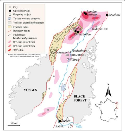
Fig. 1 Simplified geological map of the Upper Rhine Graben indicating the geothermal gradients and status of current deep geothermal fields (modified from the final report of the GeORG Project INTERREG IV 2013)
