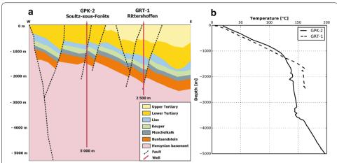
**Fig. 2** a East–West simplified vertical section of the Rhine Graben crossing the Soultz-sous-Forêts GPK–2 and the Rittershoffen GRT-1 wells (from Edel et al. 2018); **b** temperature logs, at equilibrated thermal conditions, for the Soultz-sous-Forêts GPK-2 well (from Genter et al. 2010) and for the Rittershoffen GRT-1 well (from Baujard et al. 2017) (vertical scale is in MD)
