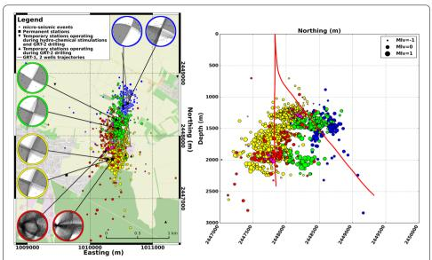
**Fig. 13** Epicenter map (left) and South–North vertical projection (right) of the seismicity recorded during the development of the Rittershoffen deep geothermal site: GRT-1 drilling (magenta circles), thermal stimulation (red circles), hydraulic stimulation (yellow circles), burst of seismicity (green circles) and GRT-2 drilling (blue circles). Focal mechanisms have been computed for two representative events for each seismogenic period (except for GRT-1 drilling)
