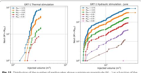
**Fig. 11** Distribution of the number of earthquakes above a minimum magnitude ( $M_{Min}$ ) as a function of the injected volume for the thermal stimulation (left) and hydraulic stimulation (right)
