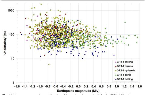
**Fig. 14** Hypocenter uncertainty as a function of the earthquake magnitude for the GRT-1 drilling (magenta circles), thermal stimulation (red circles), hydraulic stimulation (yellow circles), burst of seismicity (green circles) and GRT-2 drilling (blue circles). Please note the logarithmic scale of the vertical axis
