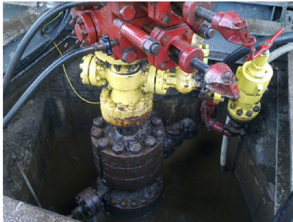
Fig. 12 Lower part of the original Poręba Wielka IG-1 wellhead together with a flange connection to the casing head (photo: B. Bielec)
