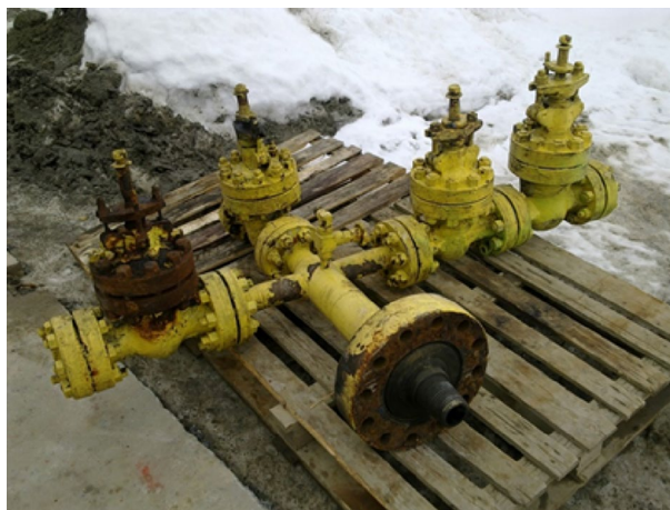
Fig. 11 Dismantled old wellhead of the Poręba Wielka IG-1 well (photo: B. Bielec)
