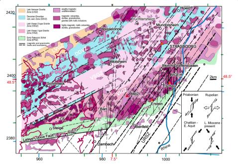
**Fig. 9** Interpretative map of the magnetic and gravimetric data with expected basement lithologies, petrographic discontinuities and faults. See details in Fig. 8. URSZ: Upper Rhine shear zone. BIGEH: Bois d'Illkirch-Graffenstaden-Eschau Horst. Inset: schematic tectonic model of the investigated area during Cenozoic times (after Villemin and Bergerat 1987)
