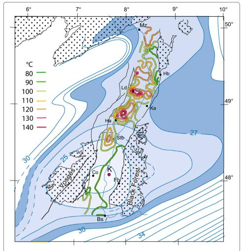
**Fig. 2** Temperature distribution at 2000 m TVD, interpolated from borehole measurements of the Upper Rhinegraben (Baillieux et al. 2013) and topography (in km) of the Moho derived from refraction and reflexion seismic sections (e.g., Edel et al. 2006). K is the 17 Ma Kaiserstuhl volcano
