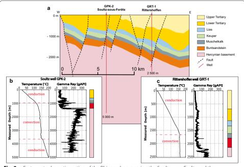
**Fig. 3** a East–west schematic section of the Rhinegraben crossing the Soultz-sous-Forêts and the Rittershoffen wells. Gamma ray and temperature log at equilibrated thermal conditions between surface and 5 km depth, **b** in the Soultz-sous-Forêts well, and **c** in the Rittershoffen well
