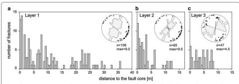
**Fig. 7** Fracture orientation and intensity in Cleebourg, shown for three individual layers. In layers 1 and 2, the fracture orientations are comparable and the fracture intensity increases towards the fault core. In layer 3, fracture orientation and intensity show a different pattern. Rose diagrams with equal area scaling and 10° bin size and equal area pole point plots on the lower hemisphere
