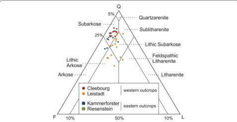
**Fig. 3** Modal composition of sandstone samples from the different locations in a QFL diagram, after McBride (1963). The sandstone compositions of Leistadt, Riesenstein, and Kammerforster are adopted from Soyk (2015)
