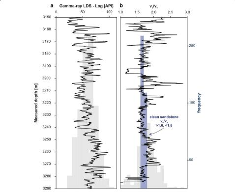
**Fig. 10** Vertical bore logs of lithological and mineralogical properties and the corresponding histograms. **a** Results from LDS gamma-ray log, implying reduced API values in the middle of the reservoir. **b** Ratio of  $\nu_5$  and  $\nu_p$  wave velocities, used to determine the purity of the reservoir sandstone. Typical values for sandstone are marked in blue
