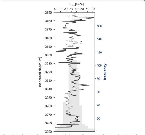
**Fig. 12** Vertical variation of Young's modulus with histogram. The grey dotted lines show data rejected due to bad hole conditions. The calculation is based on density and compressional  $(v_p)$  and shear  $(v_s)$  wave velocities, as shown in Fig. 11a, c)
