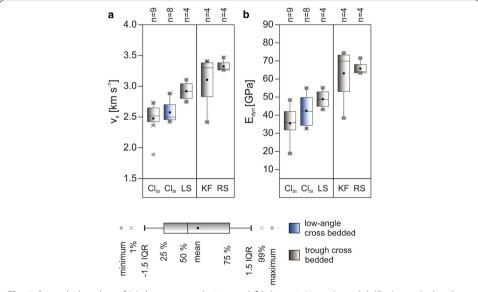
**Fig. 5** Box–whisker plots of (**a**) shear-wave velocities and (**b**) dynamic Young's moduli ( $E_{\rm dyn}$ ), as calculated from sonic velocities. Outcrops ordered according to their location, from west to east, and colour coded according to fabric type
