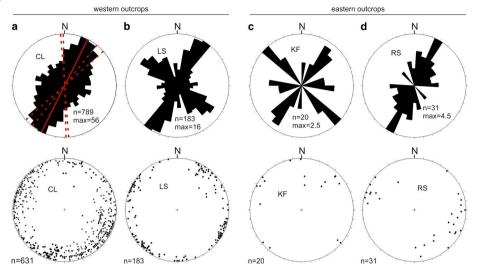
**Fig. 6** Fracture orientation data shown in equal area-scaled rose diagrams with 10° bin size and in pole plots (equal area, lower hemisphere). **a** Cleebourg (CL) fracture orientation data with the strike of the main fault (bold line) and minor faults (dashed lines) marked, **b** Leistadt (LS), **c** Kammerforster (KF), and **d** Riesenstein (RS)
