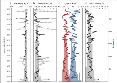
**Fig. 11** Vertical bore logs of rock properties and the corresponding histograms. **a** The bulk density as calculation basis for (**b**) the bulk porosity. **c** The compressional wave velocities (and additionally the shear-wave velocities) on the basis of calculation for (**d**) the matrix porosity. The grey dotted lines show data rejected due to bad hole conditions
