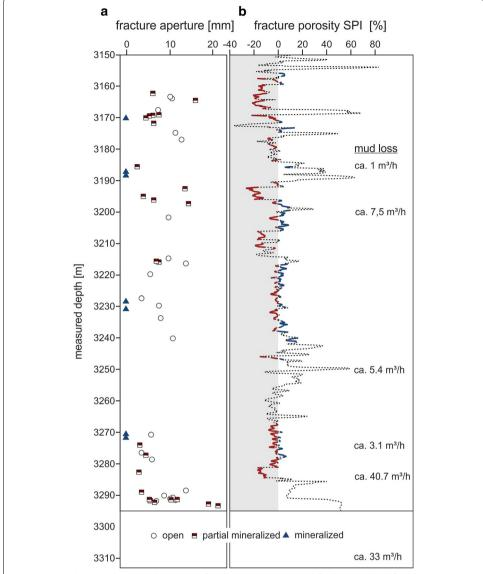
**Fig. 14** Plots showing the vertical variation of (a) fracture aperture and (b) the calculated fracture porosity (secondary porosity index), and observed mud loss during the drilling operation, as a proxy for the structural permeability. The grey dotted lines show rejected data, e.g. data found to be biased by bad hole conditions, red bold lines negative and blue bold lines positive fracture porosities
