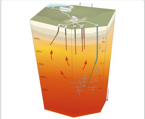
**Fig. 1** Conceptual model of the Reykjanes geothermal field showing the existing conventional geothermal wells (*brown*) and the IDDP-2 well (*blue*) (Friðleifsson et al. 2016)
