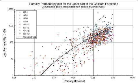
**Fig. 8** *Plot* of core analysis data from a local field. The porosity–permeability *plot* is based on core samples from selected Stenlille gas storage facility wells. The data are measured on horizontally orientated plug samples. Data originate from the main reservoir section, i.e. the upper part of the Gassum formation. Note the *scattered data*. The Stenlille trend line (*black*) is calculated without applying any cut-offs. *ST* Stenlille
