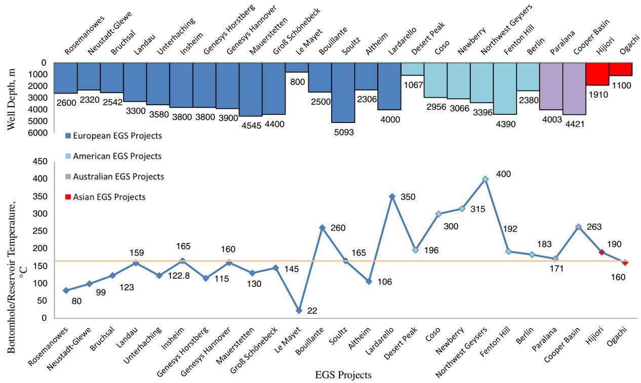
**Figure 1** Worldwide EGS projects' reservoir/bottomhole temperature vs. depth.
