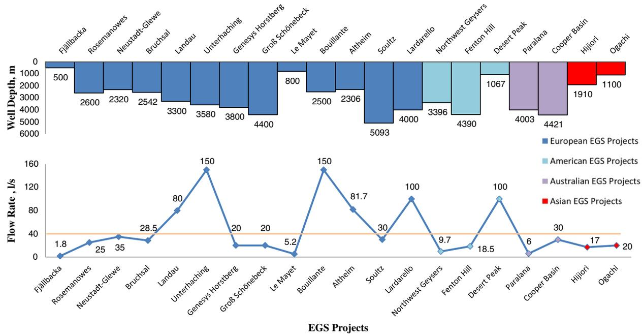
Figure 2 Worldwide EGS projects' flow rate vs. depth.
