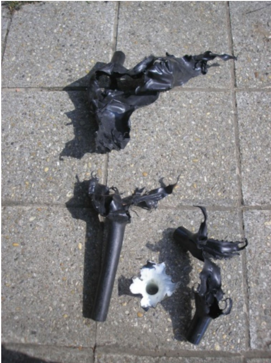
Fig. 9 Experimentally ruptured PE pipe, left from the Semtex charge, right from the pyrotechnic charge
