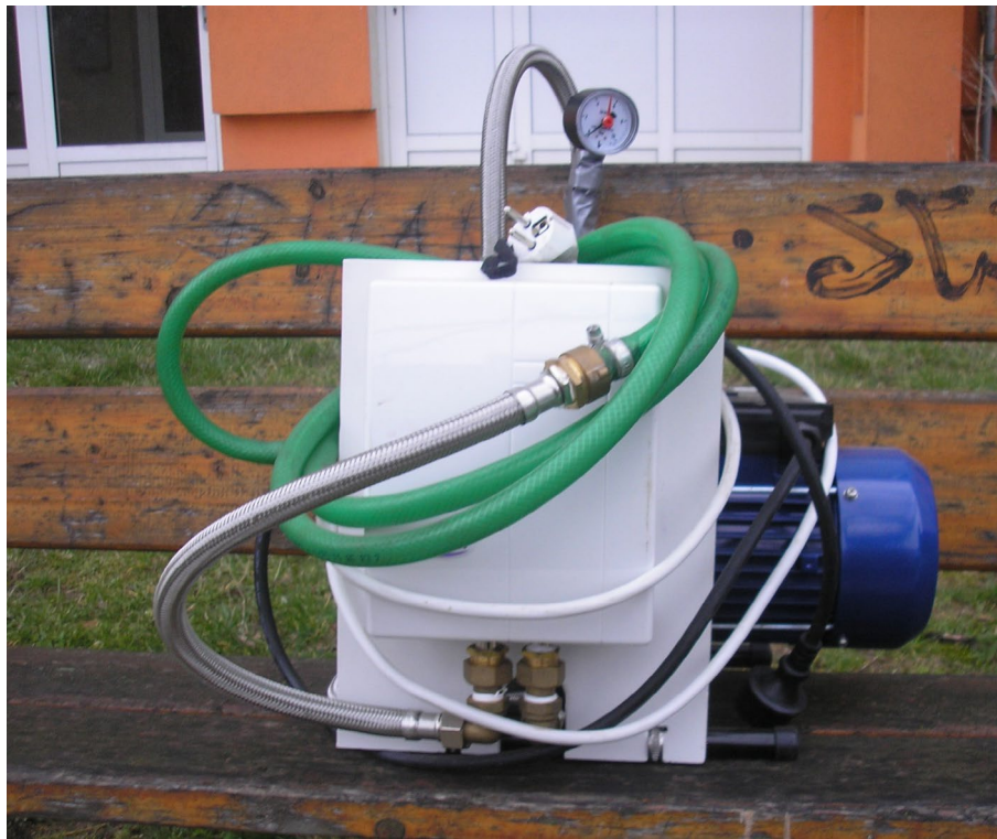
Fig. 7 Induction thermometry device with a heat output of 3 KW
