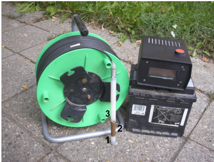
Fig. 4 Small diameter probe on GGL. 1: emitter; 2: shielding; 3: detector
