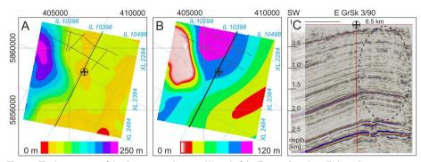
**Fig. 17** Thickness maps of the Quaternary deposits (**A**) and of the Tertiary Rupelton (**B**) based on Stackebrandt and Manhenke (2010). Superimposed in grey lines are the mapped main faults in the upper Zechstein (this study) and the orientation of the seismic profile shown in **C**. **C** Seismic section of the pre-stack depth migration volume with CRS stack after depthing (profile D in Fig. 6) showing less continuity of seismic reflectors in the stippled area
