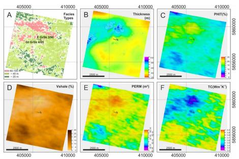
**Fig. 14** Analysis of the Elbe reservoir sandstone (ERS) derived from reservoir and seismic modelling. **A** Seismic facies types in the EBS according to Bauer et al. (2020), **B** Thickness map of the EBS (unit 3 in the geological model. Average property maps of the EBS showing total porosity (PHIT, **C**), shale content (Vshale, **D**), permeability (mD, **E**), and thermal conductivity (TC, **F**). Superimposed are the borehole paths of the GrSk boreholes (black lines in panel centres)
