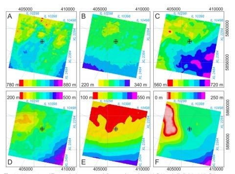
**Fig. 10** Mesozoic and Tertiary thickness maps. **A** Buntsandstein (M3–X1), **B** Muschelkalk (M1–M3), **C** Keuper (L4–M1), **D** Jurassic (BLC–L4), **E** Cretaceous (based on Stackebrandt and Manhenke (2010) and the mapped BLC horizon), **F** Tertiary (mainly based on Stackebrandt and Manhenke (2010), combined with borehole data). The cross marks the location of the E GrSk 3/90 borehole
