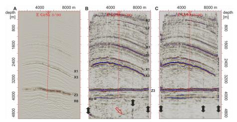
**Fig. 6** Depth-converted seismic sections along NW–SE trending profile B (for location see Fig. 7). **A** Post-stack time migration without CRS stack, **B** pre-stack depth migration with CRS stack, **C** pre-stack depth migration with multiple reduction (see also Table 1). Black arrows indicate processing artefacts; the red arrow marks a multiple reflection
