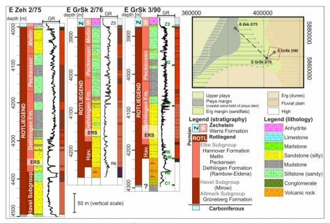
**Fig. 2** Rotliegend in East Brandenburg (Groß Schönebeck) as encountered in selected boreholes (interpreted from drilling reports) and respective facies interpretation according to Doornenbal and Stevenson (2010; inset map). ERS marks the sedimentary geothermal target (Elbe reservoir sandstone). GR are gamma-ray log readings for correlation (partly digitized)
