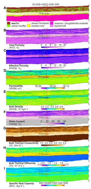
**Fig. 13** Facies (**a**) and petrophysical parameterization (**b–i**), assuming a thickness of the volcanic sequence of about 200 m. Shown are 6.5 km long W–E cross sections covering the central part of the seismic survey in the depth range of 3800–4400 m, located approximately 75–200 m north to the Groß Schönebeck boreholes (views from the south). Exaggeration: approximately 1.5
