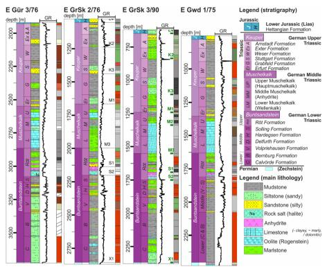
**Fig. 3** German Triassic deposits (thickness, lithological composition, and prevailing rock colour) as encountered in boreholes in East Brandenburg, interpreted from unpublished drilling reports. For location of boreholes, see Fig. 1. GR are gamma-ray log readings for correlation (partly digitized)
