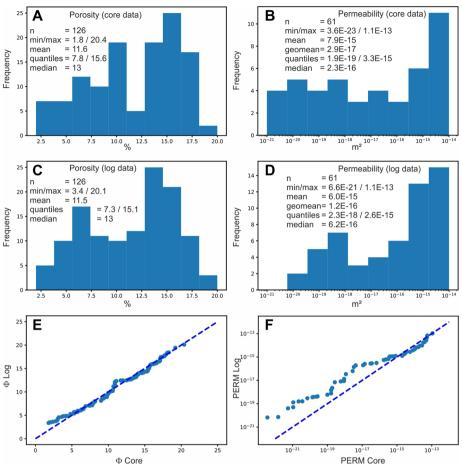
**Fig. 12** Histograms (**a**–**d**) and quantile–quantile plots (**e**, **f**) of total porosity (in %) and permeability (in mD) for core data (**a**, **b**) and corresponding log-based data (**c**, **d**) for the stream floodplain facies of the EBS (E GrSk 3/90)
