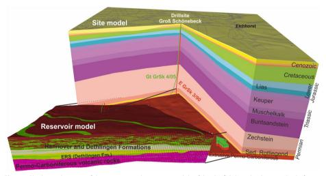
**Fig. 15** Block visualizations of the new site and reservoir models of the Groß Schönebeck research platform, view from south. The size of the site model is  $10 \, \text{km} \times 10 \, \text{km}$ , the size of the reservoir model 6.5 km  $\times$  6.5 km
