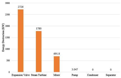
Fig. 2 Bar chart of splitting exergy destruction rates of components
