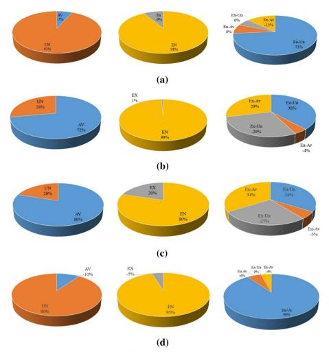
Fig. 4 Splitting exergy destruction rates of components: a Expansion valve, b steam turbine, c pump, and d mixer
