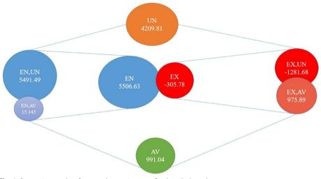
Fig. 6 Separation results of exergy destruction rates for the whole cycle
