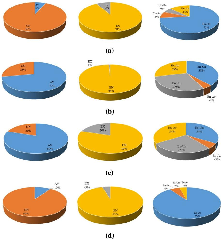
**Fig. 4** Splitting exergy destruction rates of components: **a** Expansion valve, **b** steam turbine, **c** pump, and **d** mixer
