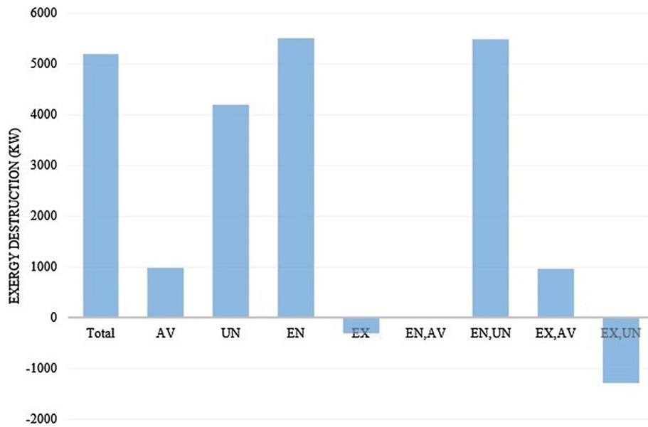
**Fig. 5** Bar chart of different parts of exergy destruction for all the system
