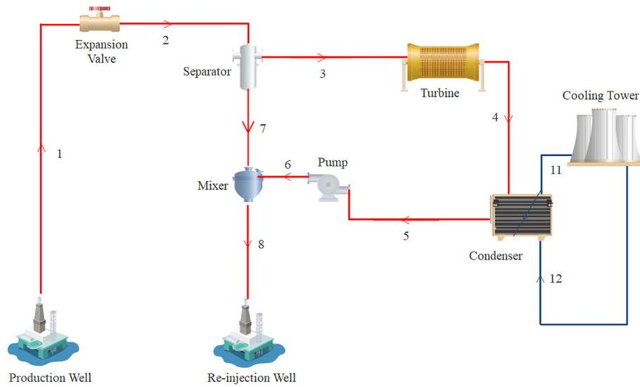
**Fig. 1** Single flash geothermal cycle diagram
