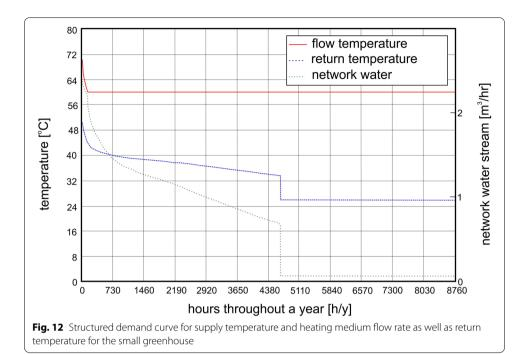
For a small greenhouse facility with a cubature of 98,000 m<sup>3</sup> the maximum power requirement of a single facility was estimated at 51.6 kW for heating, 2.7 kW for hot water preparation and 535 GJ/y for total heat demand. The heating characteristics for such a facility are presented in Figs. 11 and 12.
