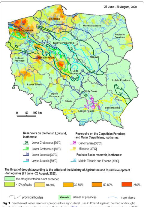
**Fig. 3** Geothermal water reservoirs proposed for agricultural uses in Poland against the map of drought threats. Scientific description based on Barbacki et al. (2016); ranges of reservoirs with temperatures > 30 °C and > 60 °C according to maps by Górecki et al. (2006, 2011, 2012, 2013); Map of drought threats according to ISSPC-NRI (2020)—sample data from 21 June to 20 August, 2020
