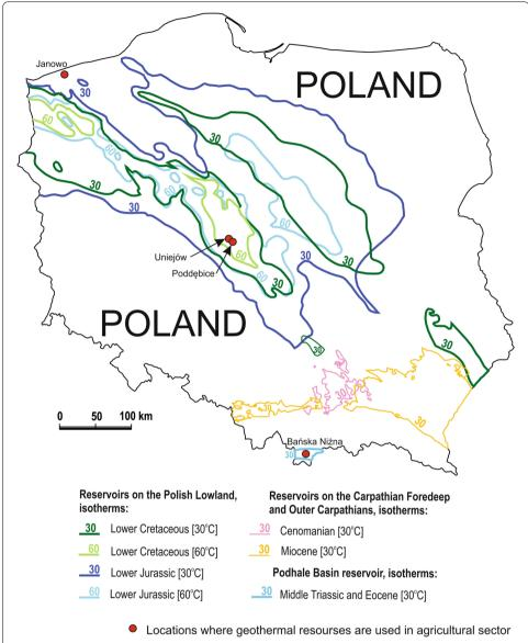
**Fig. 1** Map of geothermal water reservoirs proposed for agricultural uses in Poland. Scientific description based on Barbacki et al. (2016); ranges of reservoirs with temperatures > 30 °C and > 60 °C according to maps by Górecki et al. (2006, 2011, 2012, 2013)
