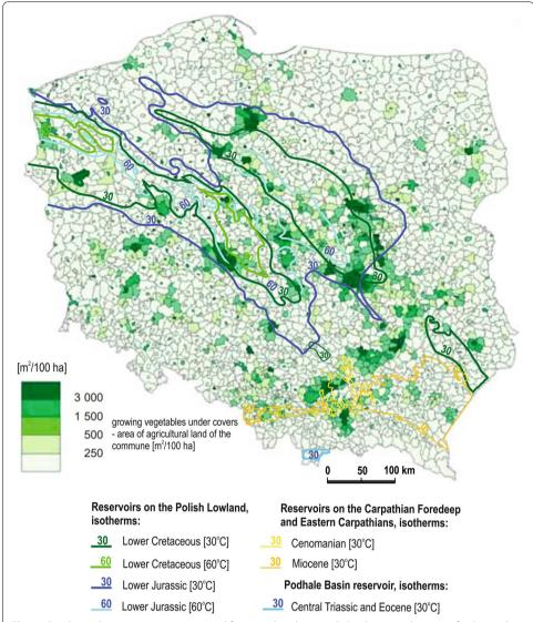
**Fig. 8** Geothermal water reservoirs proposed for agricultural uses in Poland against the map of cultivated vegetables under covers. Scientific description based on Barbacki et al. (2016); ranges of reservoirs with temperatures > 30 °C and > 60 °C according to maps by Górecki et al. (2006, 2011, 2012, 2013); underlay Map of vegetables crops under cover (2002 [in:] Kulikowski 2007)
