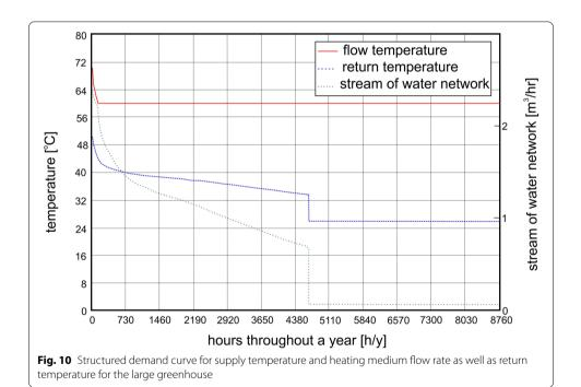
figure shows that a complete (qualitative–quantitative) control of the power delivered was assumed. As the temperature of the geothermal water is not high, quantitative control (consisting in adjusting the required water stream to the greenhouse's requirements) is of dominant importance.
