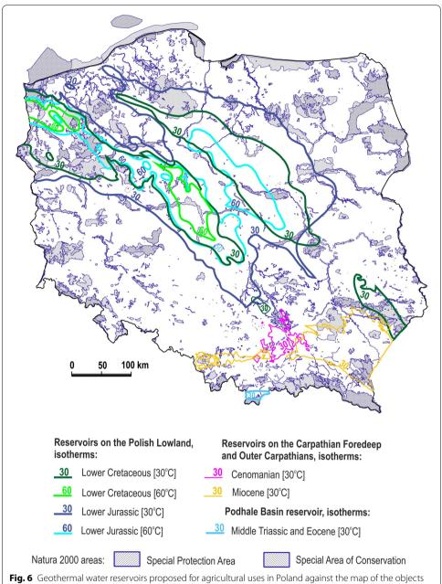
**Fig. 6** Geothermal water reservoirs proposed for agricultural uses in Poland against the map of the objects of the European Network Natura 2000 areas. Scientific description based on Barbacki et al. (2016); ranges of reservoirs with temperatures > 30 °C and > 60 °C according to maps by Górecki et al. (2006, 2011, 2012, 2013); underlay the Map of the Nature 2000 areas (GDEP 2021; HOGC 2021b)
