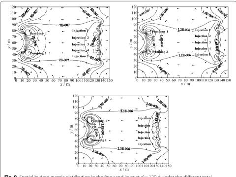
**Fig. 9** Spatial hydrodynamic distribution in the fine sand layer at d=120 d under the different total pumping–injection flow volume  $\sum G$ : **a**  $\sum G=200$  m<sup>3</sup> d<sup>-1</sup>; **b**  $\sum G=600$  m<sup>3</sup> d<sup>-1</sup>; **c**  $\sum G=1200$  m<sup>3</sup> d<sup>-1</sup>
