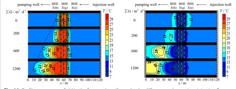
**Fig. 10** Profile temperature field in the fine sand aquifer under the different total pumping–injection flow volume: **a** the end of the cooling stage (120 d); **b** the end of the heating stage (300 d)
