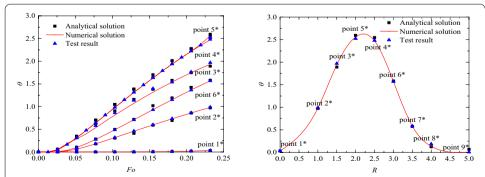
**Fig. 6** Comparison of multi-tube (four-tube) analytical solution and numerical solution with experimental result (y=0 m, z=0.5 m): **a** temperature response  $\theta$  over Fo (the observation points  $1*\sim6*$ ); **b** temperature response  $\theta$  over dimensionless distance L (Fo = 0.232)
