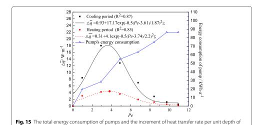
which shows that  $\Delta \bar{q}$  is distributed as a Gaussian function with the uptrend of Pe (Fig. 15). Although the effect of convective heat transfer and thermal dispersion between the BHEs and the rock—soil layer can be enhanced effectively by strengthening the velocity of groundwater seepage, the average heat transfer rates per unit borehole depth of the BHEs (q) does not raise linearly with the increase of the pumping—injection flow volume.
