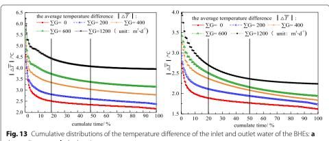
the cooling stage; **b** the heating stage
