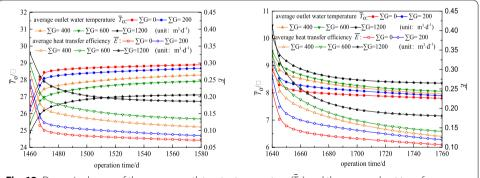
**Fig. 12** Dynamic change of the average outlet water temperature  $(\bar{T}_o)$  and the average heat transfer efficiency  $(\bar{E} = \bar{Q}/\bar{Q} = |\bar{T}_i - \bar{T}_o|/|\bar{T}_i - \bar{T}_{S_0}|)$  of the BHEs in the fifth operation cycle: **a** the cooling stage; **b** the heating stage
