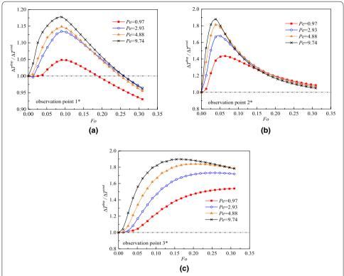
**Fig. 11** Temperature response dynamic curve in the fine sand aquifer at the first cooling stage: **a** the upstream area of the BHEs (the observation point 1\*); **b** the inside area of the BHEs (the observation point 2\*); **c** the downstream area of the BHEs (the observation point 3\*)
