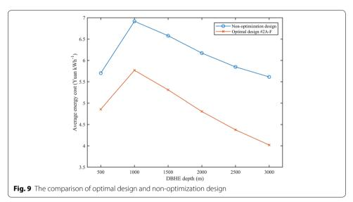
Lukawski et al. 2014, 2016). Therefore, in our cases, a DBHE of 3000 m should be the most economical choice when one wants to get the maximum heat with the lowest cost. In addition, Fig. 8 shows that the AEC value is similar when DBHE depth is 500 and 2000 m, which means the economic benefit of building a 2000 m DBHE is similar to build 4 DBHEs of 500 m. In this case, it is sure one 2000 DBHE is more economical than 4 DBHEs of 500 m due to the lower area demanding.
