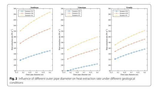
simulated the outlet temperature and heat transfer capacity under different outer pipe diameters. The results demonstrate that the outlet temperature and heat transfer capacity both increase with an increase to the outer pipe diameter. Because this study is concerned with changes in the optimal heat extraction rate, the trend of heat extraction rate in our study is different from the trend of outlet temperature in Wang et al. (2017).
