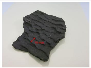
**Fig. 1** Ripple scale sample collected from the inlet of the heat exchanger. The sample has a calcite composition. Some oil contained in the thermal water is incorporated in the scale causing the black color. The shape of the ripples with a luv and lee side points to current flow ripples
