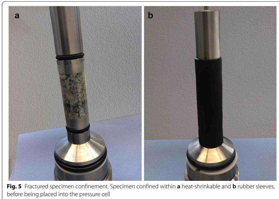
**Fig. 5** Fractured specimen confinement. Specimen confined within **a** heat-shrinkable and **b** rubber sleeves, before being placed into the pressure cell
