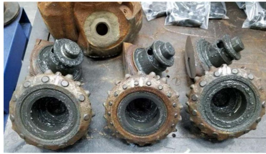
Fig. 6 Cones and bearing from high-temperature tri-cone roller cone drill bits used during drilling of the IDDP-2 well in the Reykjanes geothermal field in Iceland (Stefánsson et al. 2018)
