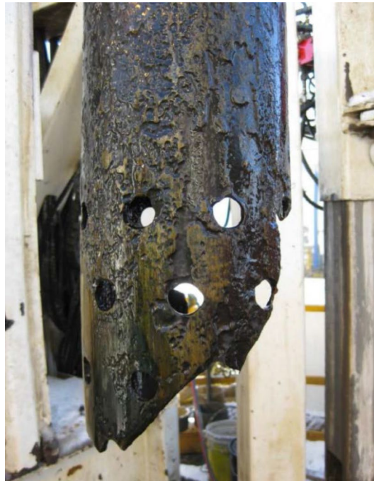
Fig. 3 Heavy corrosion of liner pipe in the KJ-39 well (source: deliverable D4.3 from GeoWell project, Thorbjörnsson 2016)
