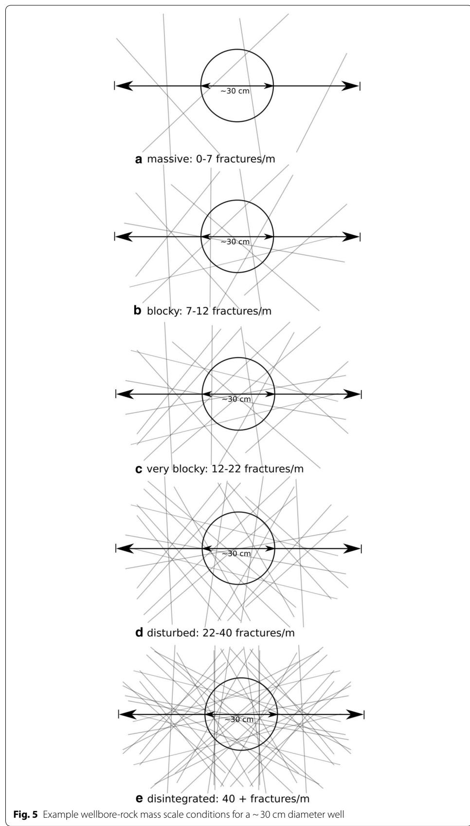
**Fig. 5** Example wellbore-rock mass scale conditions for a ~ 30 cm diameter well
