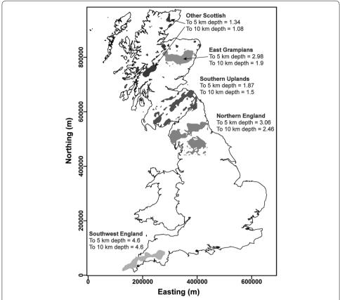
**Fig. 3** Locations in Great Britain with significant quantities of heat producing granites within the upper crust. Quantitative figures of average heat production in,  $\mu$ Wm<sup>-3</sup>, are shown for depths to 5 and 10 km respectively
