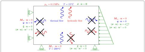
**Figure 8 Schematic representation of the boundary conditions used in the simulation.** Red, hydraulic; blue, thermal; green, mechanical. The ruled arrows represent the thermal and hydraulic flows.  $\sigma_{xx}^{reg}$  corresponds to the regional stress, see Equation (32).
