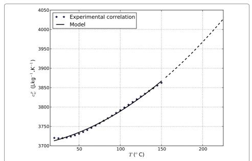
Figure 3 Correlation comparison of Equation (16) with that of Zaytsev and Aseyev (1992). Comparison of Equation (16) (plain and dotted lines) with the correlation of Zaytsev and Aseyev (1992) (data points) evaluated for a NaCl mass fraction w = 0.1.
