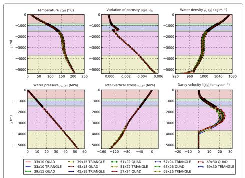
**Figure 10 Calculated vertical profiles.** Calculated vertical profiles for different mesh refinements and two kinds of finite elements (triangle and quad). The notation  $n_X \times n_y$  indicates the number of quad elements used in the two directions of the mesh. The different background colors correspond to the geological layers considered in the model.
