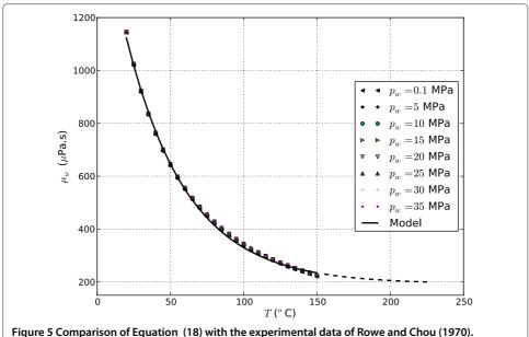
Figure 5 Comparison of Equation (18) with the experimental data of Rowe and Chou (1970).
