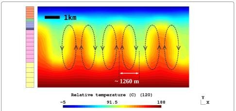
**Figure 11 Calculated relative temperature field for a mesh.** Mesh size is 10 km in width and 5.3 km in height. The relative temperature corresponds to the real temperature minus 20°C. The dotted circular lines indicate the appearance of convective cells, and the colored vertical legend indicates the width of geological layers.
