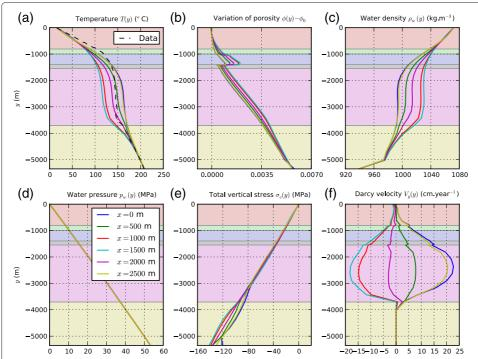
**Figure 7 Calculated vertical profiles obtained every 500 m for** *x* **between 0 and 2,500 m.** The different background colors correspond to the geological layers considered in the model. **(a)** Temperature. **(b)** Variation of porosity. **(c)** Water density. **(d)** Water pressure. **(e)** Total vertical stress. **(f)** Darcy velocity.
