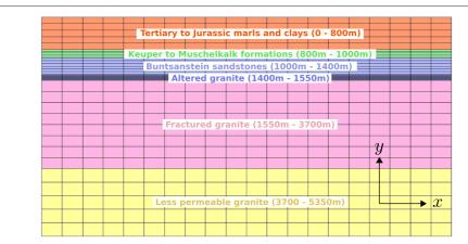
**Figure 6 Idealized cross section of the Soultz-sous-Forêts reservoir.** The reservoir is 10 km in width and 5.3 km in height and is meshed with quad elements. Each color corresponds to a geological layer.
