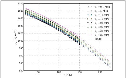
Figure 1 Experimental correlation comparison of Equation (15) with that of Rowe and Chou (1970). Comparison of Equation (15) (plain and dotted lines) with the experimental correlation of Rowe and Chou (1970) (data points) evaluated for a NaCl mass fraction w = 0.1.
