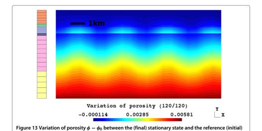
state. Model of 10 km in width, 5.3 km in height. The vertical colored legend indicates the width of
