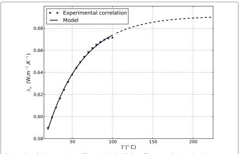
Figure 4 Correlation comparison of Equation (17) with that of Zaytsev and Aseyev (1992). Comparison of Equation (17) (plain and dotted lines) with the correlation of Zaytsev and Aseyev (1992) evaluated for a NaCl mass fraction w = 0.1.
