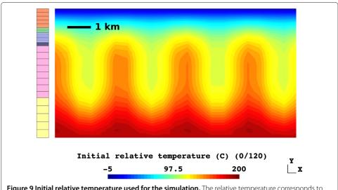
**Figure 9 Initial relative temperature used for the simulation.** The relative temperature corresponds to the real temperature minus 20°C. The colored vertical legend indicates the width of geological layers (5.3 km in height).
